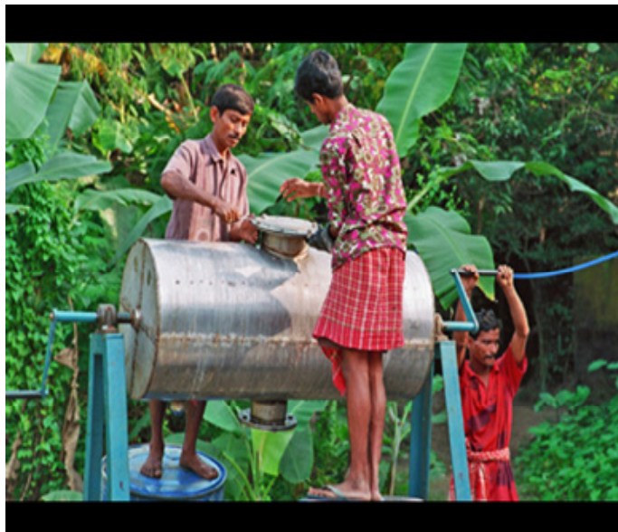
Centralized Regeneration Facility - a WFP project in India used to remove arsenic from drinking water
